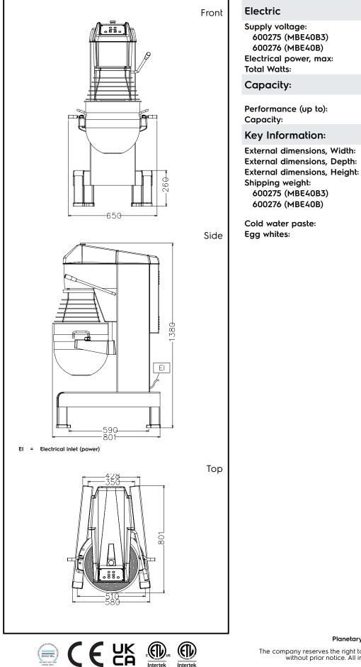
380-480 V/3 ph/50/60 Hz 200-240 V/1N ph/50/60 Hz 2.2 kW 2.2 kW
